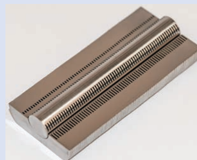
Figure 6: Laminated Object Manufacturing (LOM) of heat exchangers, filters and reformers by diffusion bonding of plates containing chemically-etched channels
