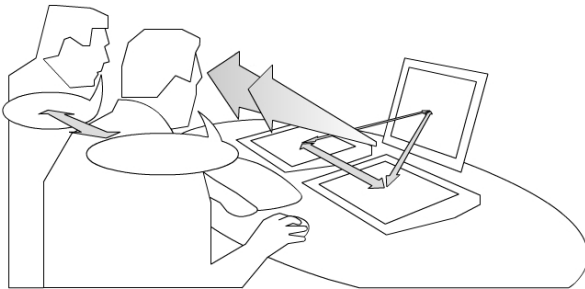
Figure 5b An alternative shared interactional workspace, with multiple linked displays, supporting shoulder-to-shoulder interactions. It provides a shared reference that can help reduce social awkwardness and improve coordination.
