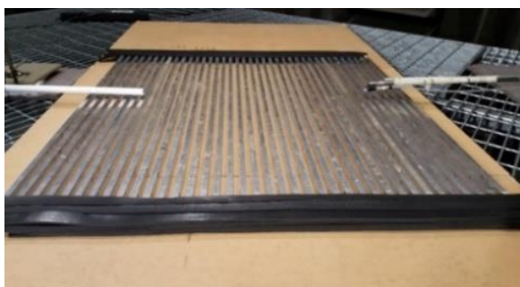
Figure 3. A laboratory arrangement of an array of 30 × 1 m long parallel aluminium strips (height 0.025 m, width 0.0122 m, edge-to-edge separation 0.015 m) on Medium Density Fibreboard (MDF). Strips of felt are placed along the edges of the array parallel to the source-receiver axis.
