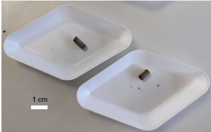
Figure 4: Strongest glycine-doped projectiles after optimising binding process - 2.9 \times 5.8 mm.
