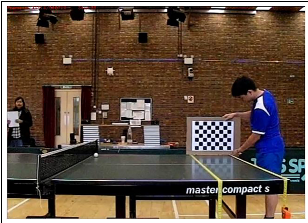
Figure 7. An upright double-sided checkerboard was used for creating reference points.
