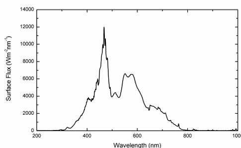
**Figure 3:** AvaSpec 2048 response to Xenon lamp.
