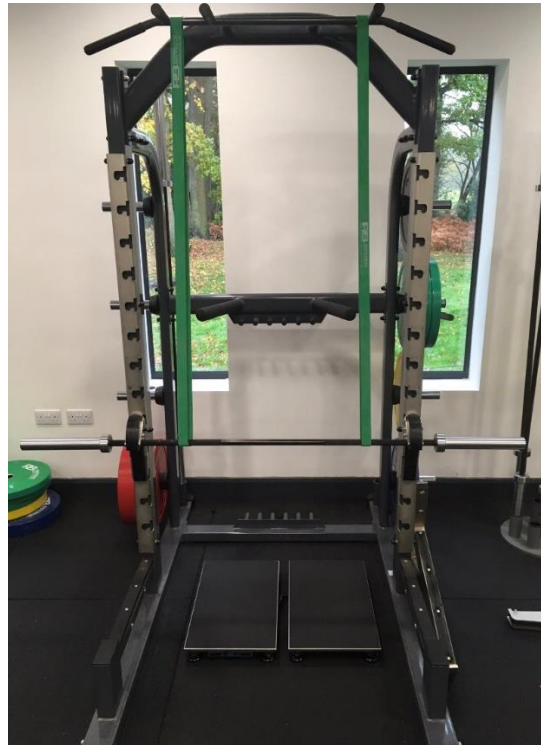
Figure 3. A gym-based set-up of an isometric mid-thigh pull.
