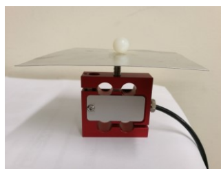
Figure 1: Load cell with attached aluminum plate; nylon sphere shown for scale
