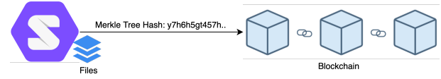
Figure 2: Storing the Merkle Tree hash of Solid pod-stored files on the Blockchain
