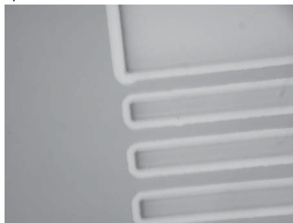
Fig. 1. Setup for undercutting measurements using optical microscope with integrated digital camera at (a) zero time and (b) after 10 min (example of Cr as sacrificial layer).
