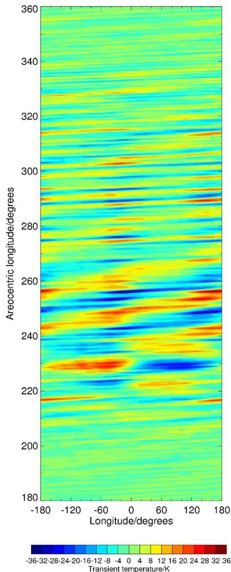
**Figure 1:** Transient temperature on the 50 Pa pressure surface ( $\sim 25$  km altitude) at  $62.5^\circ\text{N}$  over the period,  $L_S=180^\circ\text{--}360^\circ$  (northern autumnal to vernal equinox), of MY 24.
