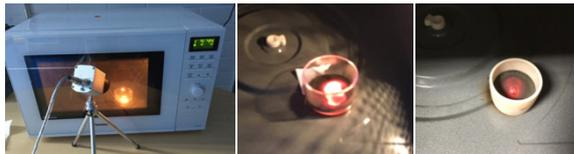
Figure 1: Microwave sintering using a kitchen microwave
