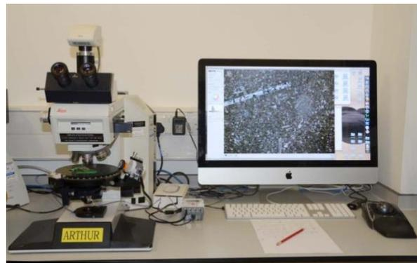
*Figure 1: Rotating stage microscope with Lego Mindstorm<sup>®</sup> motor and controller – one of two microscopes used by the virtual microscope team.*
