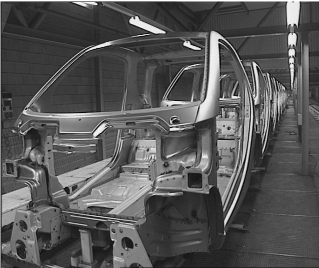
FIGURE 2: The Tridion™ safety cell, after complete assembly, by Magna Chassis, being conveyed to the main smart™ car production line.
