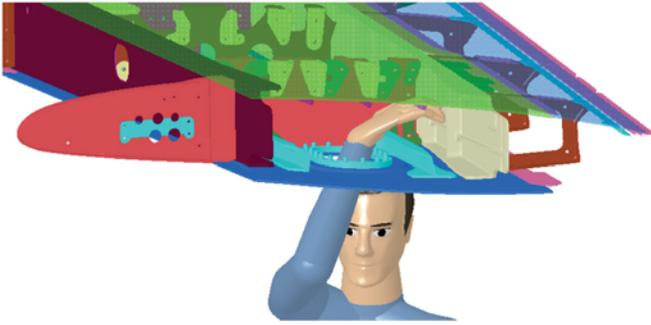
Figure 1. Example posture for wing systems installation tasks.
