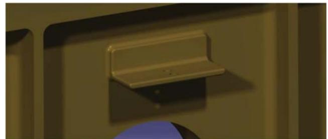
Figure 6. Integrally machined bracket
