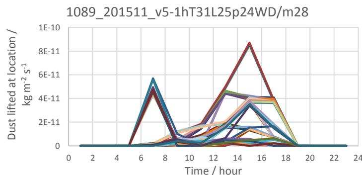
**Figure 1:** Model results of dust lifted by dust devils at the Viking Lander 2 site, showing two peaks in dust lifting at ~0900 and ~1500 local time.
