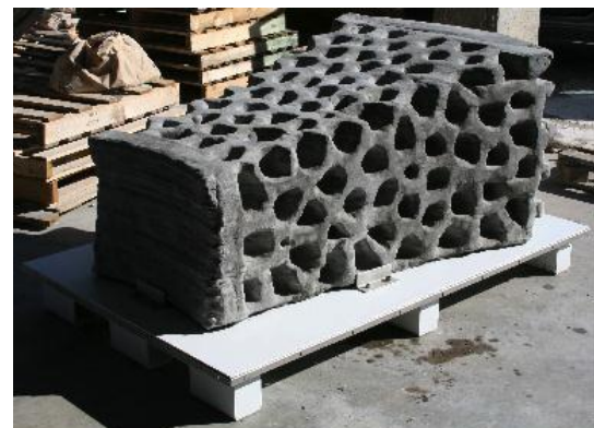
Figure 1: Printed block using a Lunar simulant (D-Shape) [22]. The approximate footprint of the block is less than 1,000 by 2,000 mm.
