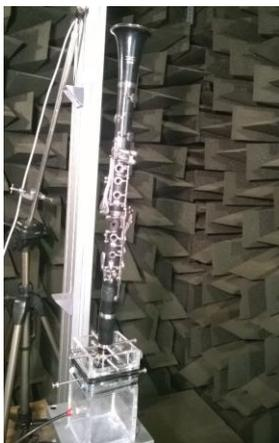
Figure 1: Artificial playing device with a clarinet
