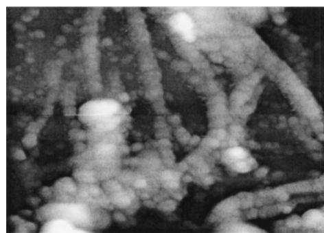
FIG. 2. AFM image ( 1 \mu\text{m} \times 0.69 \mu\text{m} ) of an annealed (800 °C) SWNT/H-Si(111) sample. The morphology of the clusterlike islands is similar to that of as-deposited SWNT aggregates.
