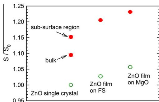
**Fig. 4.** The  $S$  parameters for ZnO crystal and thin films obtained from fitting of  $S(E)$  curves: open points – virgin samples; full points – hydrogen loaded samples. In case of ZnO (0001) single crystal the  $S$  parameter for the defected sub-surface region and for the bulk ZnO region are shown.
