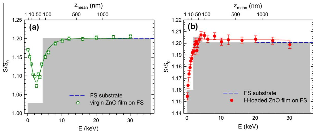
**Fig. 3.** The  $S(E)$  curves for ZnO film deposited on FS substrate: (a) virgin film (prior to deposition of Pd cap); (b) hydrogen loaded film. The mean positron penetration depth  $z_{\text{mean}}$  is shown on the upper horizontal axis. Solid lines show model curves calculated by VEPFIT software for a layered structure shown by grey areas. Dashed lines indicate the bulk  $S$  parameter for FS measured on a bare substrate.
