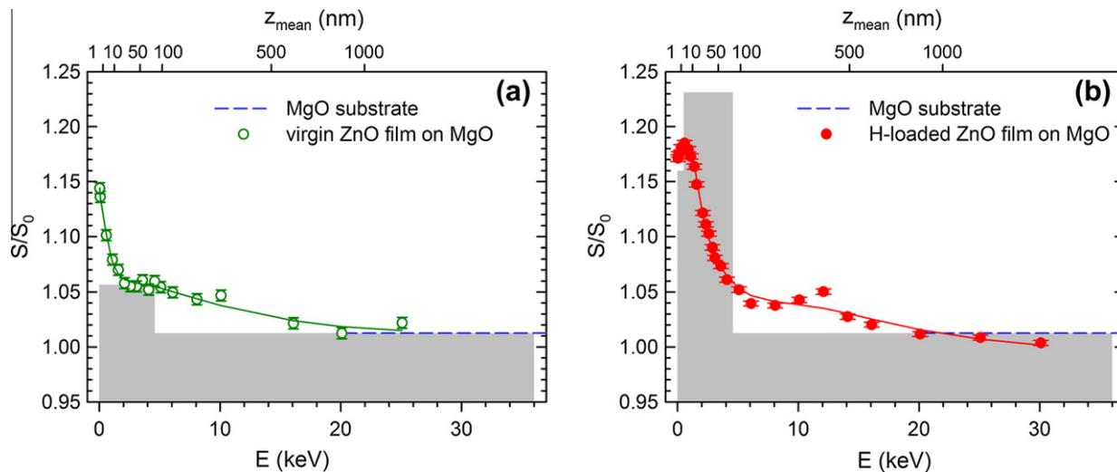
**Fig. 2.** The  $S(E)$  curves for ZnO film deposited on MgO (100) substrate: (a) virgin film (prior to deposition of Pd cap); (b) hydrogen loaded film. The mean positron penetration depth  $z_{\text{mean}}$  is shown on the upper horizontal axis. Solid lines show model curves calculated by VEPFIT software for a layered structure shown by grey areas. Dashed lines indicate the bulk  $S$  parameter for MgO measured on a bare substrate.
