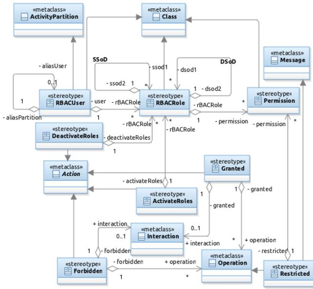
Fig. 3: Extension of the UML metamodel for rbacUML
