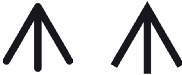
Figure 10: Broad arrows drawn to meet the proportions defined by the British Ministry of Defence Standard O5–34/2 (MoD 1984 27).
