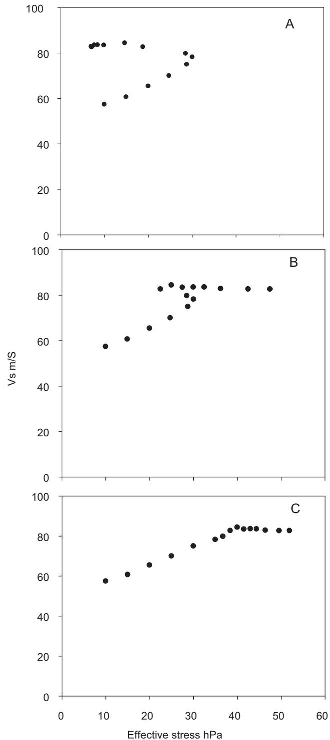
**Fig. 3.** These panels show  $V_s$  plotted against effective stress for Redhill T sand. Three different assumptions about the calculation of effective stress were made: (A)  $\chi = S$ , (B)  $\chi = S$ , if  $S > 0.5$  otherwise  $\chi = 0.5$  and (C) the function of Khallili and Khabbaz (1998).
