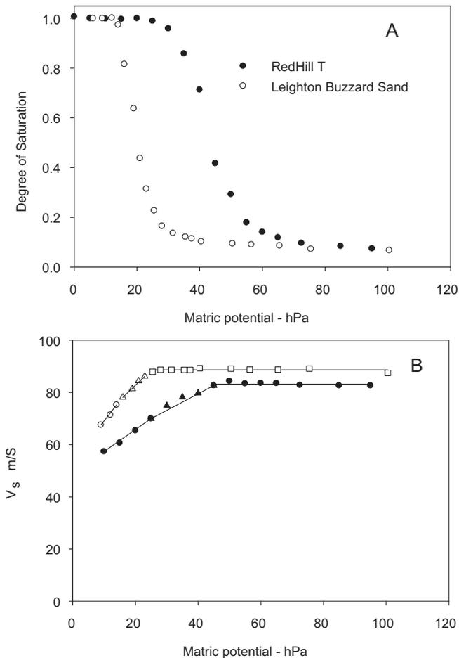
**Fig. 2.** Water retention characteristics for Redhill T and Leighton Buzzard sand are shown in the top panel. In the lower panel  $V_s$  is plotted against matric potential for these two sands. In the lower panel the three linear regions were identified visually and correspond to the regions of tension saturation, capillary fringe and residual water content.
