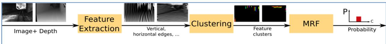
Figure 1: Architecture of the Detection System.
