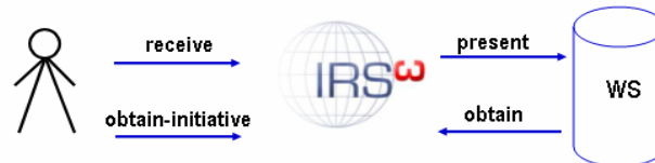
Fig. 1 A typical sequence of choreography events occurring during goal based web service invocation in IRS-III.
