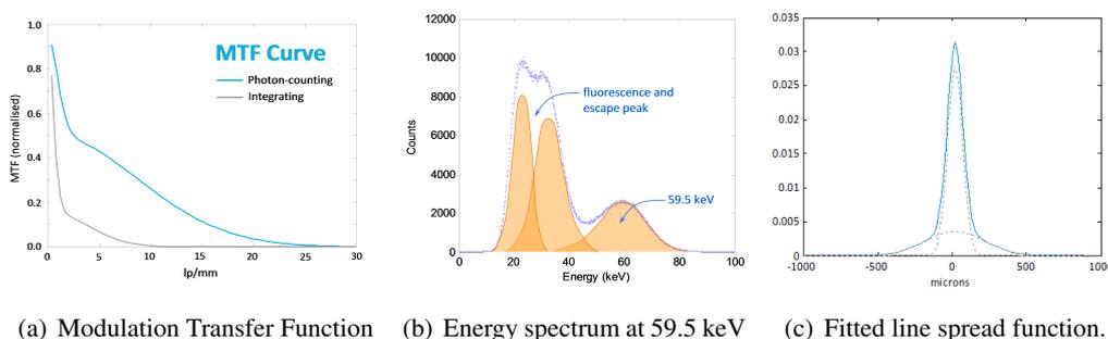
**Figure 2.** Spatial and spectral resolution measurements. The orange curves below the experimental results (blue) in the energy spectrum are given as indicators only. Adapted from [3]. The fitted line spread function (blue) is composed of two Gaussian components (grey), allowing a fit to the primary and secondary interaction components.
