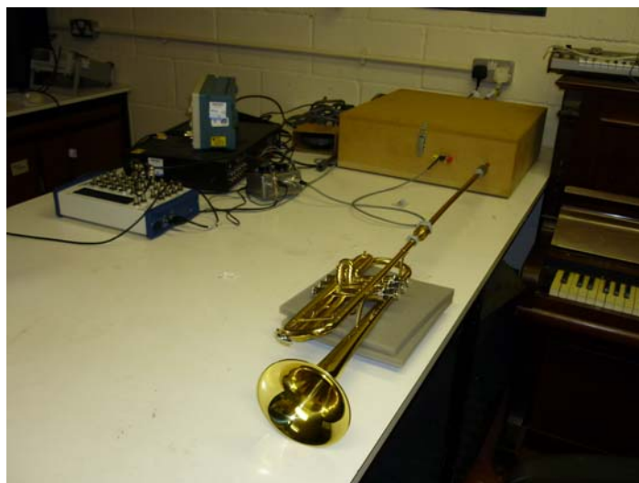
Figure 2 Acoustic pulse reflectometer coupled to trumpet
