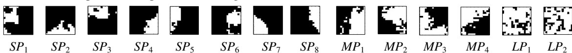
Figure 4: 64-pixel 8 small patterns (SP), 128-pixel 4 medium patterns (MP), and 192-pixel 2 large patterns (LP) are extracted using ASPS-3 algorithm from Miss America , where the white region represents 1 (motion) and black region represents 0 (no motion).
