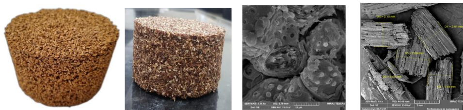
Figure 7. (left to right) cylindrical samples made from crushed walnut shells and wood chips, and FE-SEM images of walnut shell fragments (magnification 5000 \times ) and wood chips (20 \times ).
