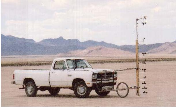
**Results:** Based on a sampling rate of 5 Hz and a typical dust column-over pass duration of one-to-four seconds, wind profiles were used to determine the surface friction speed ( $u^*$ ) and aerodynamic roughness length ( $Z_o$ ). These calculations were then compared to results obtained from nearby stationary profiling meteorology mast and field wind tunnel data [4].
