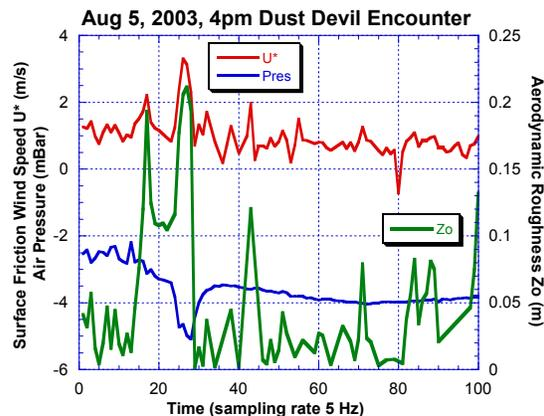
As measured by DASHER prior to the encounter,  $U^*$  on the site was 1.1 m/s and  $Z_o$  was 0.03 m. The stationary metmast results indicated the surface to have a surface roughness length ( $Z_o$ ) of 0.04 m. Wind tunnel results indicated an erosion threshold surface friction speed ( $U^*t$ ) of 1.4 m/s. During the dust devil's maximum action,  $U^*$  rose to over 3 m/s (thus making the vortex "dusty"). Note that  $Z_o$  increased by an order of
