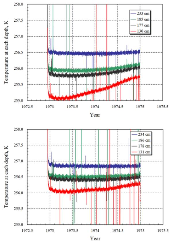
**Figure 1.** Apollo heat flow Experiment data obtained by Apollo 17 probe 1 (Upper) and 2 (Lower). As each probe has four Pt absolute thermometers, temperature profiles in time series are measured at four depth points.
