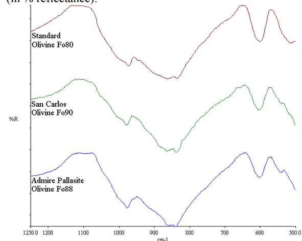
Fig.2: Diffuse reflectance FT-IR spectra of olivines from the Admire pallasite ( $\text{Fo}_{88}$ ) [4], terrestrial San Carlos olivine ( $\text{Fo}_{90}$ ) [5] (in % reflectance)
