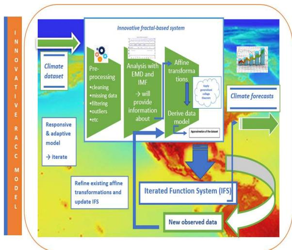
Fig. 1. Schematic of Rapid Adaptive Climate Model.
