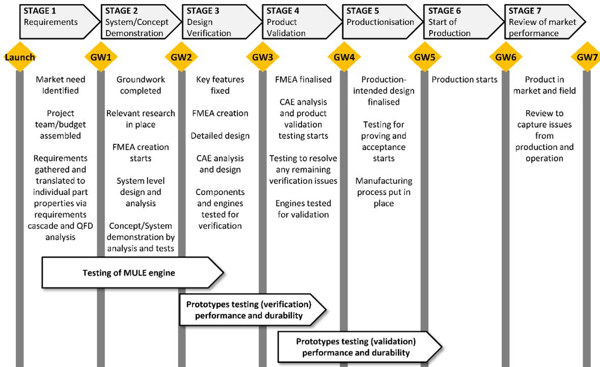
Figure 1 Stages of NPD process in the Diesel engine company.
