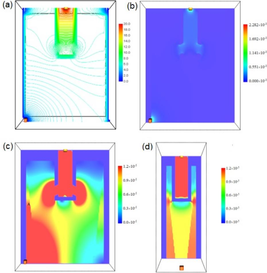
Figure 2: The distribution ( $c=0.2$ ) of (a) electric potential and (b) electric current at  $z = 0.06m$ ; rescaled current distribution at (c)  $z = 0.06m$  and (d)  $x = 0.12m$ , respectively.
