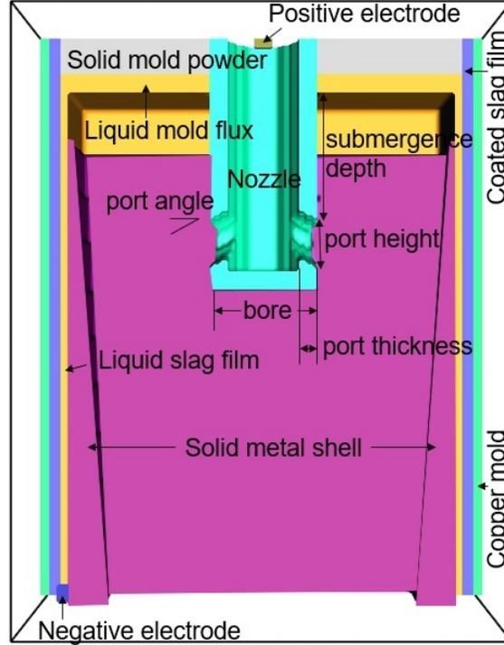
Figure 1: Schematic plotting of continuous casting mold and electrodes.
