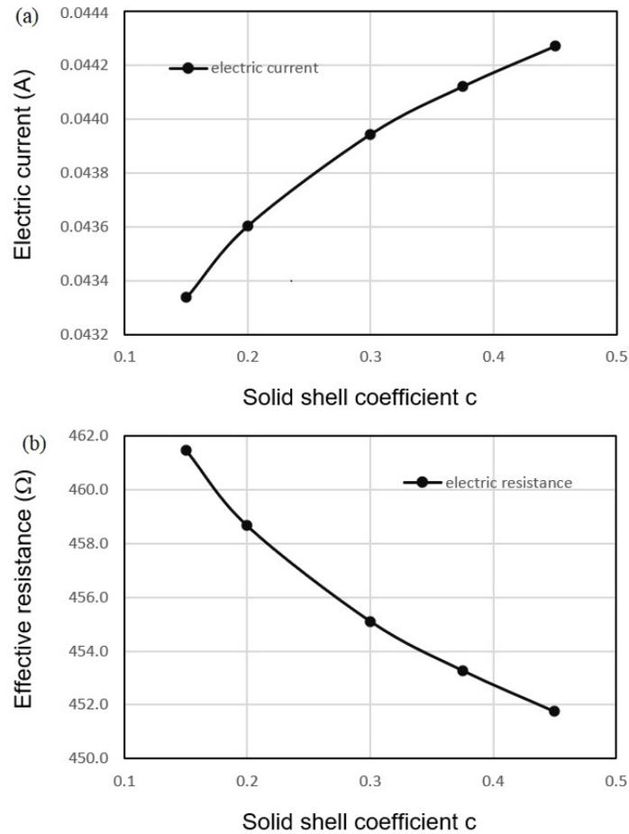
Figure 3: (a) Numerical results for electric current vs. solid shell coefficient; (b) effective electrical resistance vs. solid shell coefficient.
