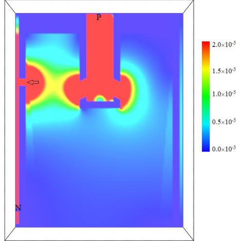
Figure 5: (a) Detection of the coating film integrity, where P, N and arrow denote the location of anode, cathode and a crack, respectively.
