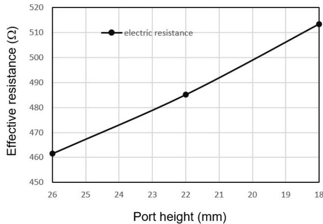
Figure 4: (a) The numerical results for the change of effective electric resistances as the port height is reduced from  $0.026m$  to  $0.018m$  due to oxide condensation.
