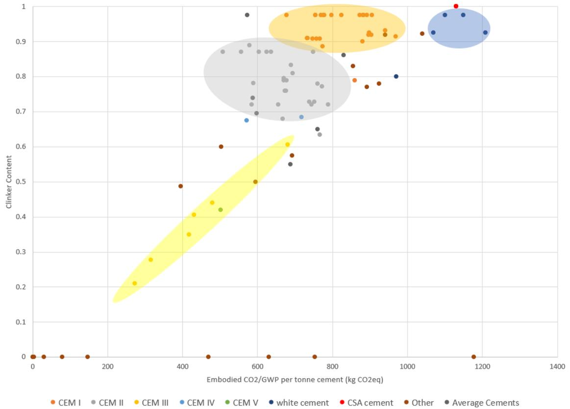
FIGURE 1. Graph showing relationship of Embodied Carbon for cements by clinker content, source [7].
