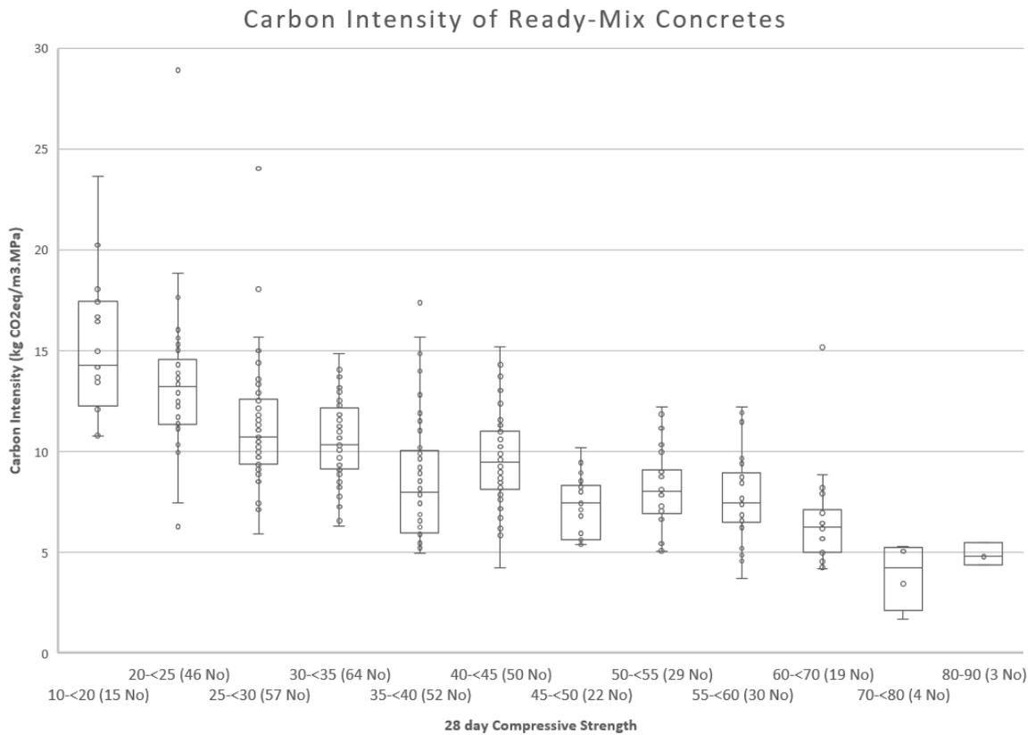
FIGURE 4. Box and Whisker Graph showing mean, upper and lower quartiles for Carbon Intensity ready-mix concretes, source [7].
