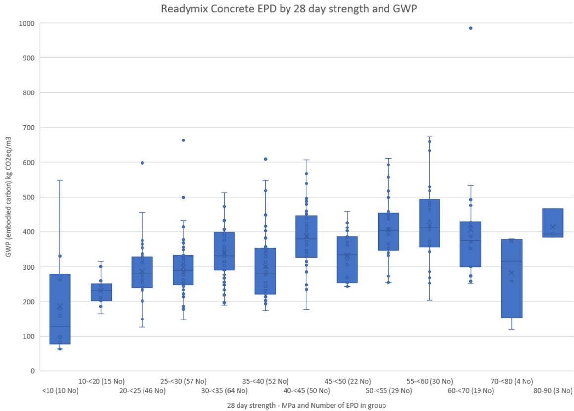
FIGURE 3. Box and Whisker graph showing mean, upper and lower quartiles of Embodied Carbon for ready-mix concretes from concrete EPD, by 28-day strength, source [7].
