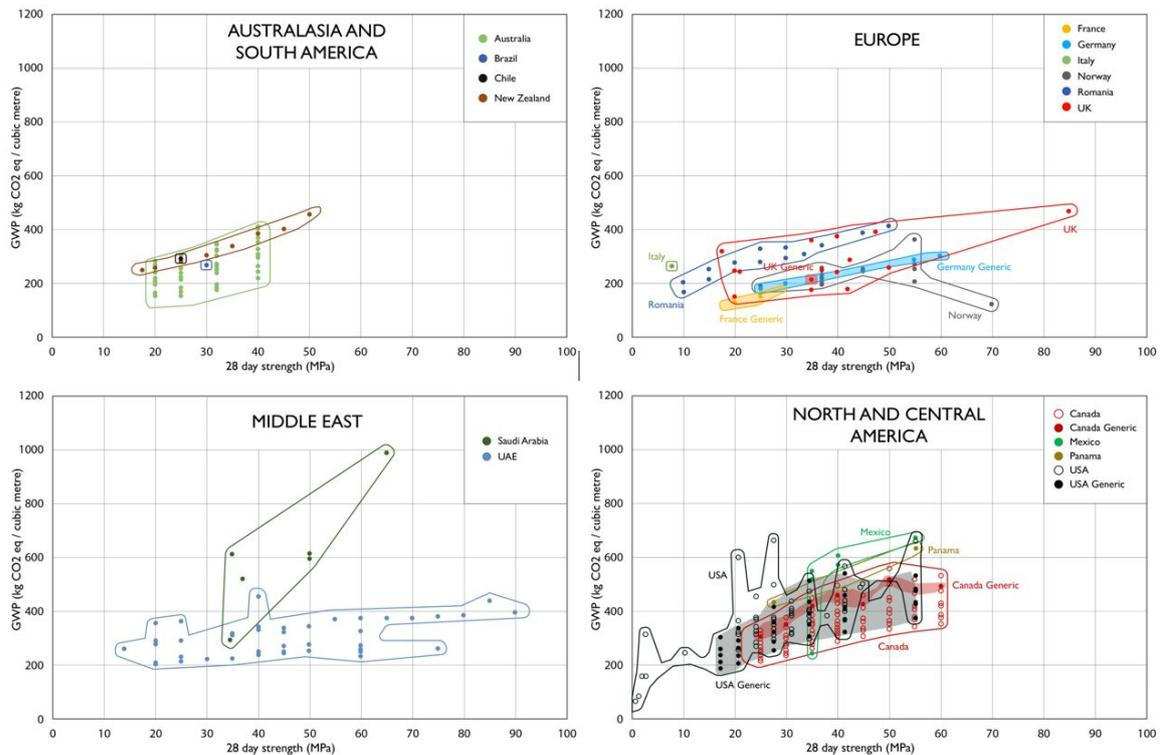
FIGURE 2. Embodied carbon per m<sup>3</sup> concrete by compressive strength, shown for each country, source [7].
