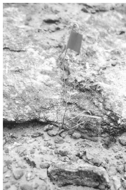
Fig. 1. Field deployment of glass slides bound with one clip and wedged apart with a second. Slides are inserted in soil or rock crevices.
