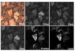
**Figure 2**: A positive dye sequence acquired using the FI on-board Zoë under ambient light conditions. This data set was taken in the Atacama Desert in the 2005 field expedition.
