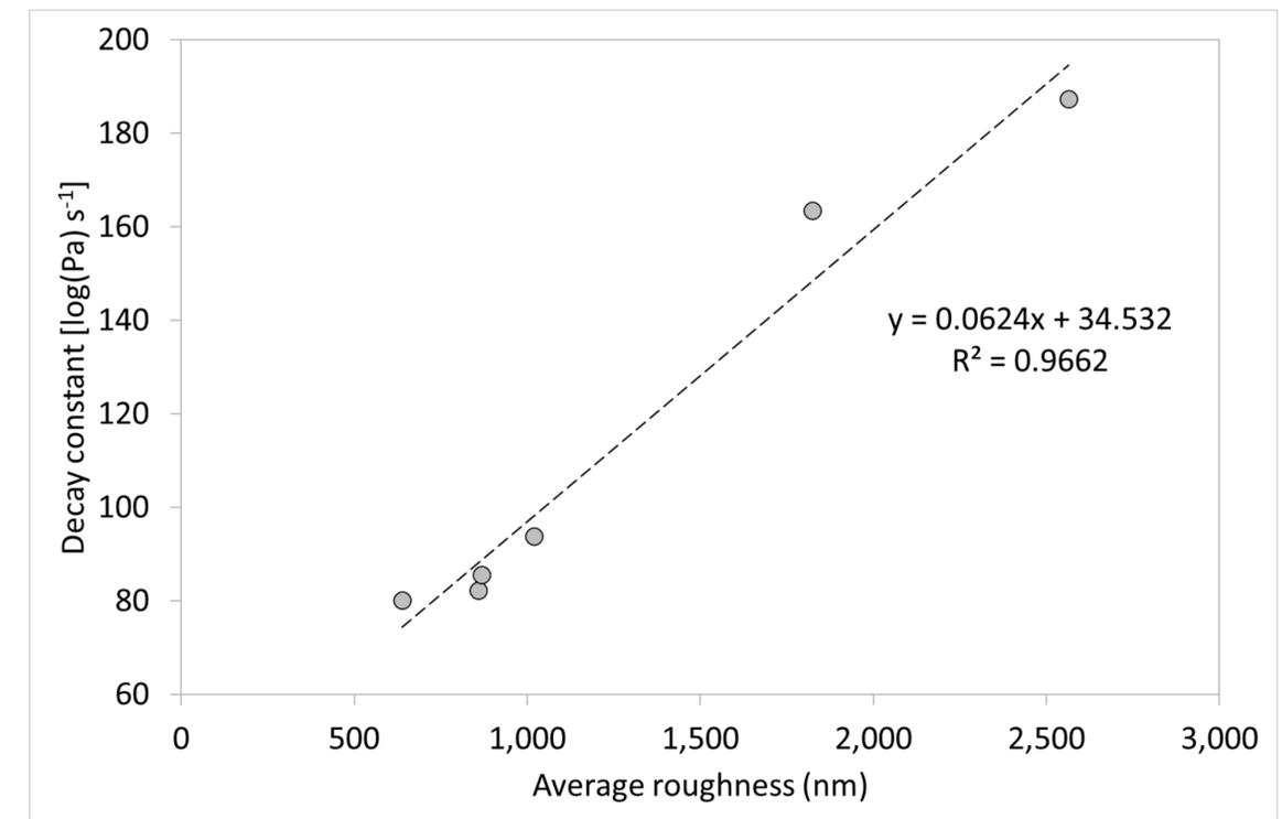
Fig 5. Effect of surface roughness on decay constant
