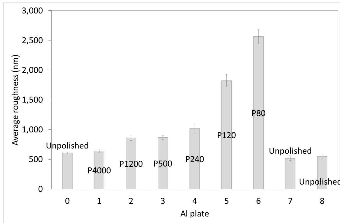
Fig 3. Average roughness of unpolished and roughened aluminium plates
