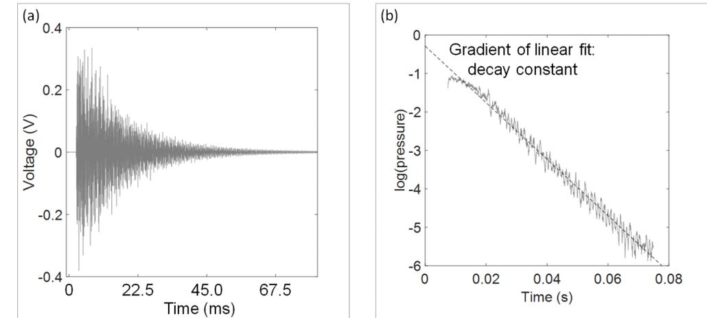
Fig 2. Sound analysis: (a) amplitude in time domain; (b) sound pressure decay
