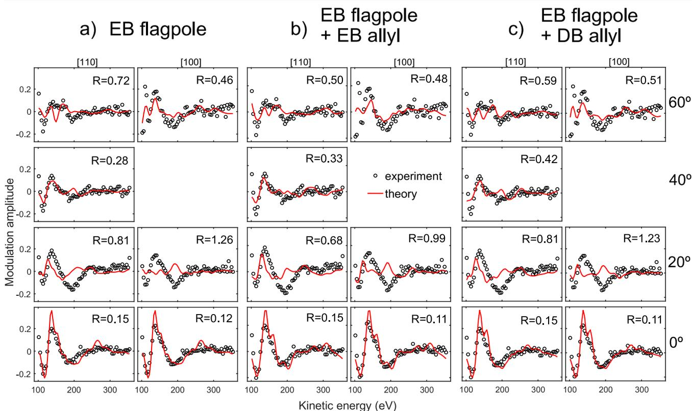
**Figure 3.** Comparison of the experimental and theoretical PhD modulations for the best fits found in the annealed preparation. Angles listed on the right-hand side are photoelectron emission angles with respect to normal emission. Inset is the individual  $R$ -factor for fit of each experimental PhD spectra to its corresponding theoretical spectra.
