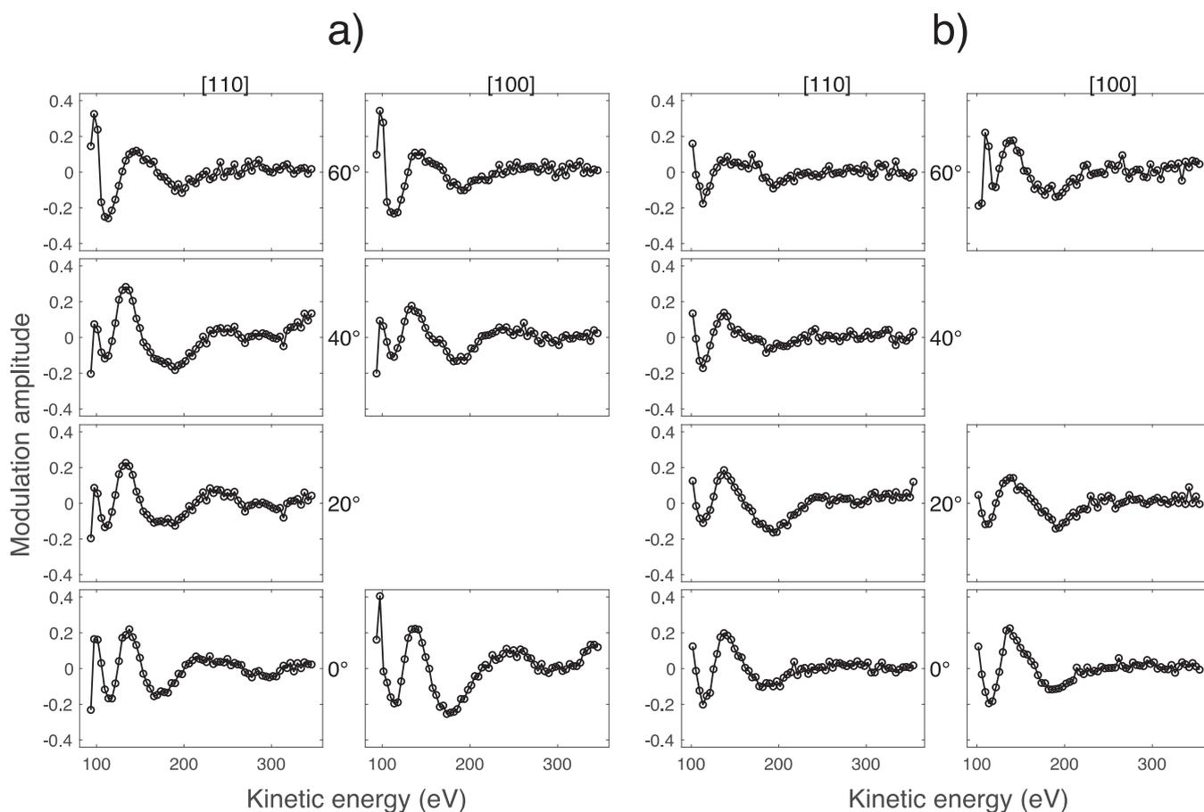
**Figure 2.** Oxygen 1s modulations amplitudes for (a) the room-temperature and (b) annealed preparation. The azimuth is shown in each column and polar emission angles with respect to normal emission in each row.
