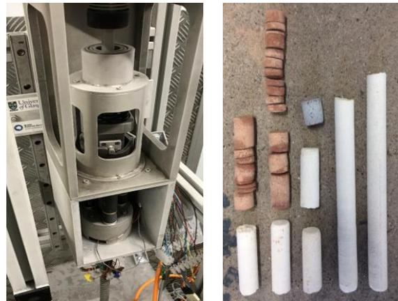
**Figure 2: P-RAID architecture (L) and core samples of sandstone, limestone and microgabbro (R)**
