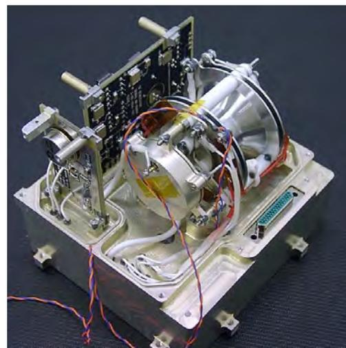
**Figure 2: The Ptolemy Ion Trap Mass Spectrometer instrument**
