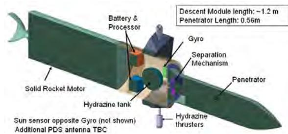
**Figure 1: High-speed penetrator de-orbit and ejection system**
