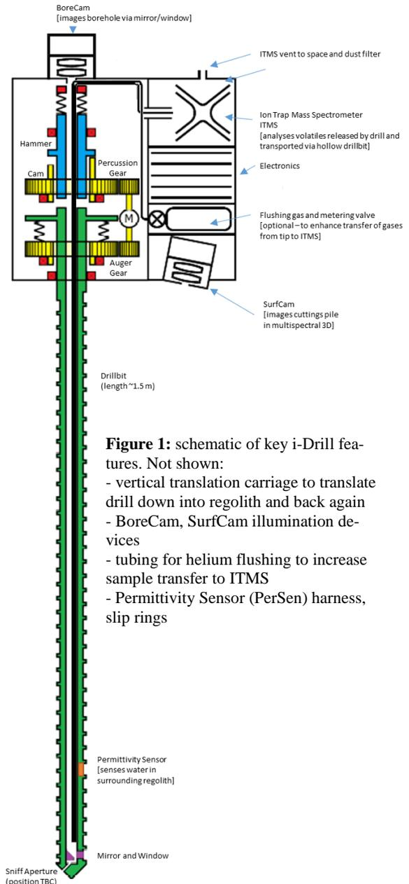
**Figure 1:** schematic of key i-Drill features. Not shown:
