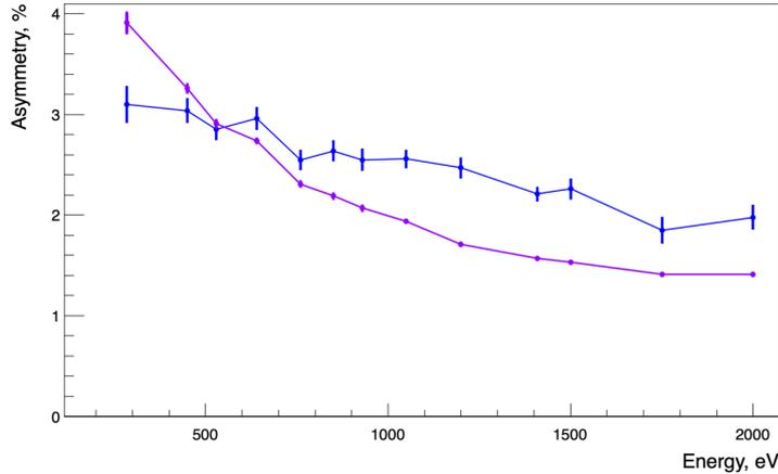
Figure 3: Average cluster central row asymmetry values for different x-ray energies.  $e_1$  - blue,  $e_2$  - magenta. Data points are connected by lines to guide the eye. (For interpretation of the references to color in this figure legend, the reader is referred to the web version of this article.)
