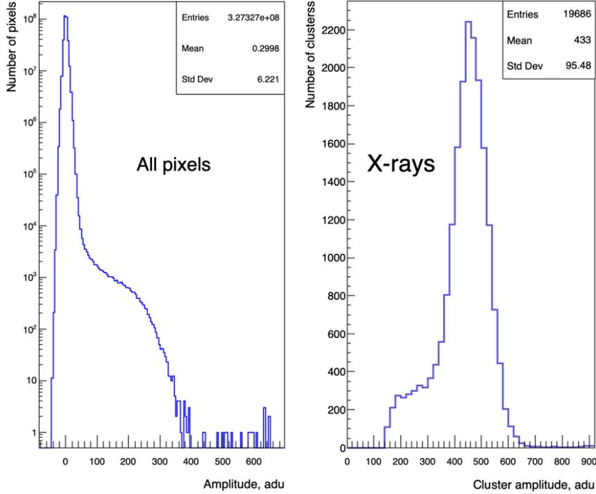
Figure 1: Pixel amplitudes and clean x-ray clusters total amplitudes at 530 eV.
