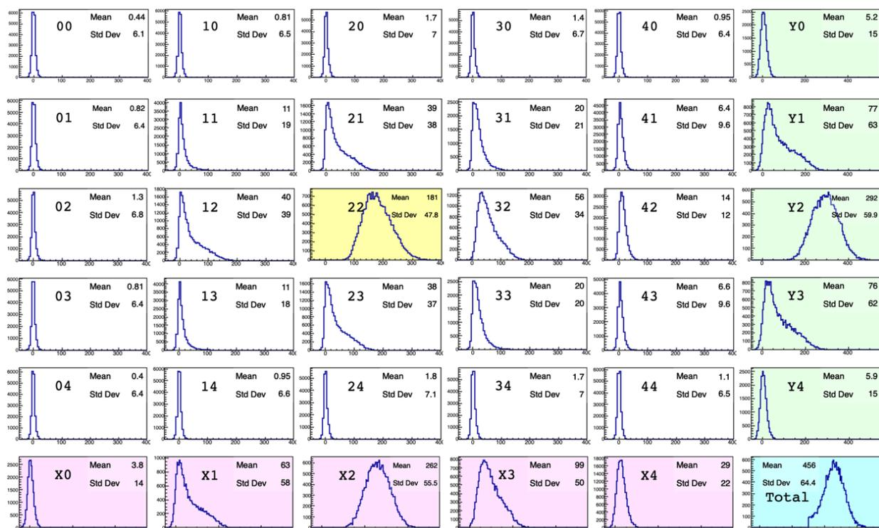
Figure 2: Amplitude distributions in  $5 \times 5$  pixel clusters and horizontal and vertical profiles. The central pixel is highlighted in yellow; vertical profile is green; horizontal profile is pink; and total sum is blue. (For interpretation of the references to color in this figure legend, the reader is referred to the web version of this article.)
