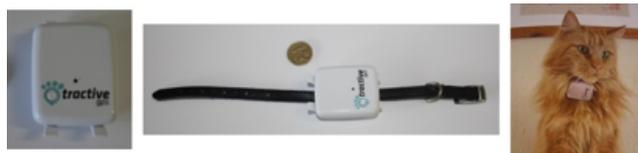
Figure 2. Tractive. Left: case. Center, collar and case (with 23mm diameter coin); Right: device on cat.
