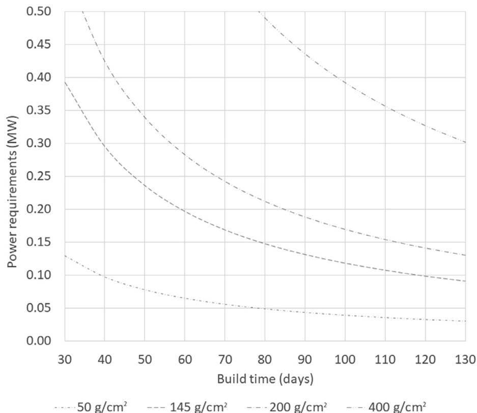
Fig. 3. Power requirements per shield thickness, as build time increases.
