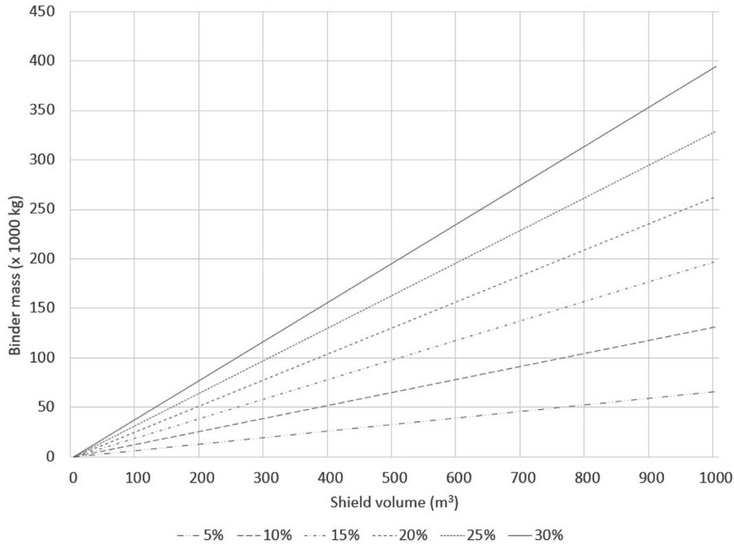
Fig. 1. Additional binder upmass per shield volume increase, using %wt values commonly found across the literature.
