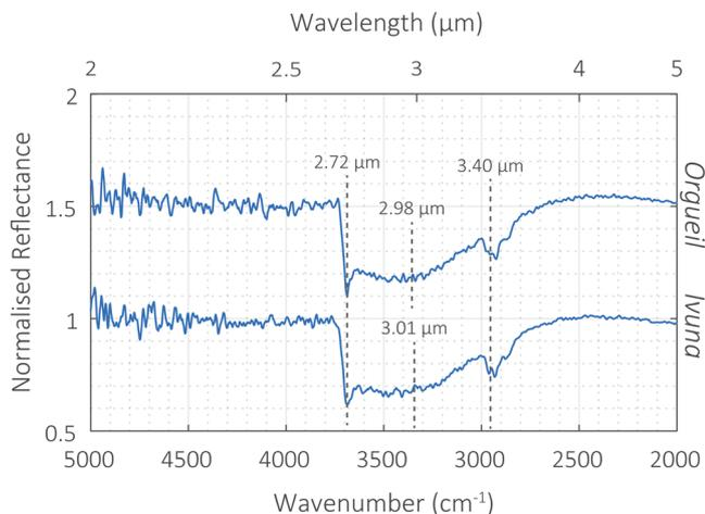
Fig. 4. The 3  $\mu\text{m}$  feature for the CI chondrites Orgueil and Ivuna. The blue spectra reflect the PSF petrologic type 1.1. Spectra are normalized to unity at 2.3  $\mu\text{m}$  and offset for clarity. There are three components to the 3  $\mu\text{m}$  feature in the CIs: at 2.72  $\mu\text{m}$  due to Mg-OH, at  $\sim 3.00$   $\mu\text{m}$  due to bound  $\text{H}_2\text{O}$ , and at 3.40  $\mu\text{m}$  due to organics.
