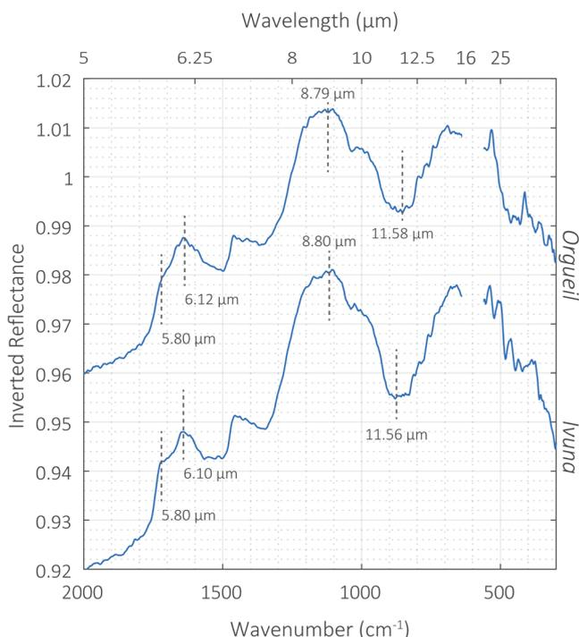
Fig. 6. MIR spectra for CI1 chondrites. The blue spectra reflect the PSF petrologic type I.1. Spectra are inverted and offset for clarity. Both spectra show similar features to the CMs; near 6  $\mu\text{m}$ , a Christiansen feature (CF) and a transparency feature (TF). These features are highlighted. The gap in the spectra is a region of low signal-to-noise due to the beamsplitter.
