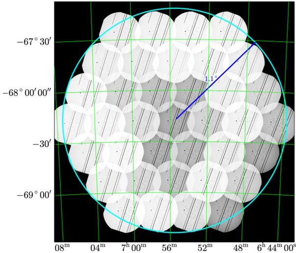
**Figure 2.** The XRT exposure map of the 37-point tiled observations of the LMC performed with *Swift*, demonstrating the structure of the pattern. The black lines are the vetoed columns on the CCD. The cyan circle has radius of 1.1 and is shown for reference. Axis are RA and Dec., J2000.
