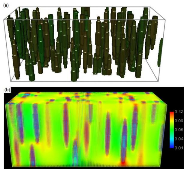
**Fig. 4.** (a) 100 rods are aligned to a direction in perpendicular to that of the electrical field and (b) the correspondence electric current density distribution.
