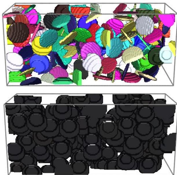
**Fig. 5.** 173 flakes in (a) random distribution and (b) aligned along the direction of electric field.
