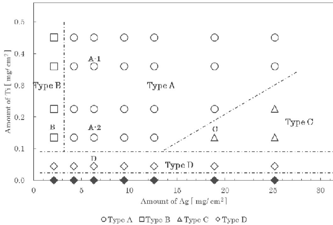
**Fig. 2. Classification of bonded copper/AlN samples based on their interfacial microstructure when using various concentrations of Ti and Ag in the brazing paste. All samples were brazed at 850 °C for 30 min under a constant pressure of 0.1 MPa**
