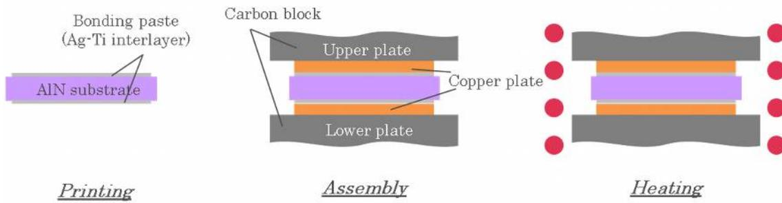
Fig. 1. Procedure used for brazing copper to AlN substrates.
